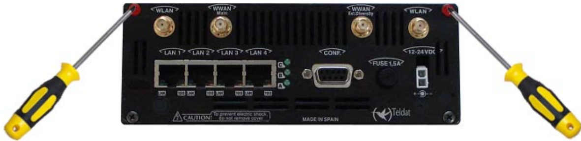
Fig. 9: Location of the screws on the front of the casing
