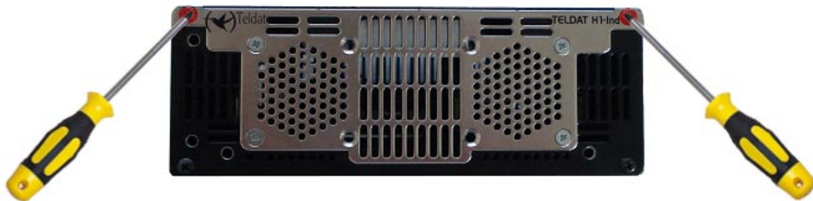
Fig. 10: Location of the screws on the rear of the casing
